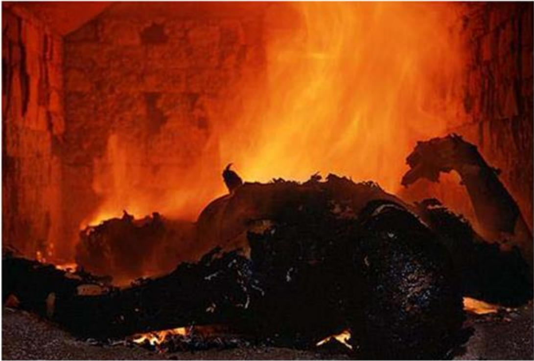
A dead body inside an industrial furnace that is able to generate temperatures of 870–980 °C (1600–1800 °F) to ensure disintegration of the corpse
